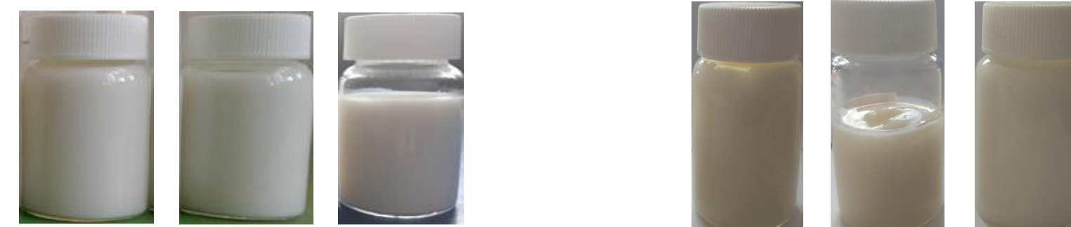
Figure 2 Stabilized emulsions: O/W:E2, E8, E10, W/O:E15, E16, E17 (4 weeks after preparation)
