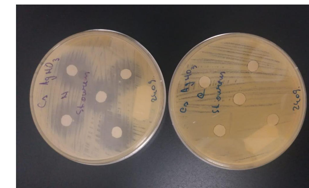
Fig .7 Antimicrobial tests result for the N and C Ag/chitosan NP treated samples
