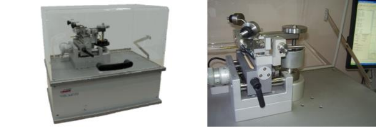
Ball-on-disk testing device in dry conditions, [1] Ball-on-disk testing device in water lubricated, [2]
