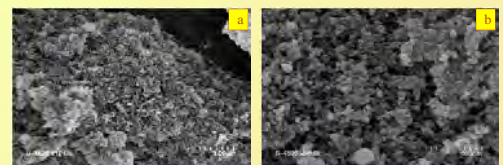
SEM images recorded for the photoluminescent aerogel (a) 10 k resolution (b) 50 k resolution
