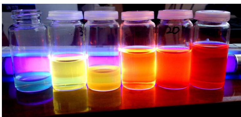
Figure 1. (left) Prepared CdSe QD's under UV excitation and (right) size distribution
