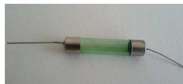
**Figure 1.** Modified PANI film on glass support
