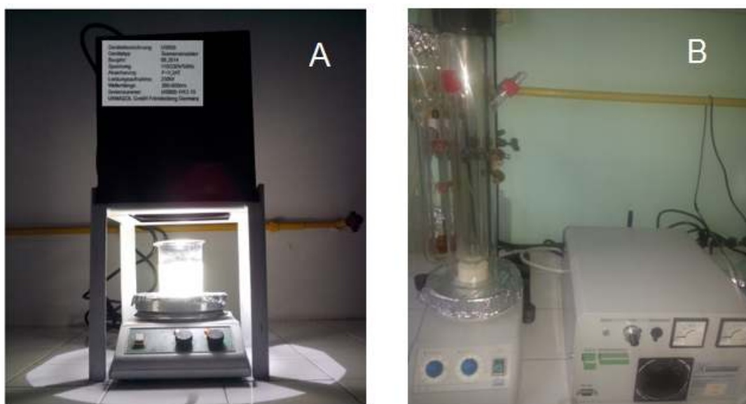
Fig1. A) The solar simulator US800(250W) B) The photo-reactor equipped with Jasco UV lamp (300 W).
